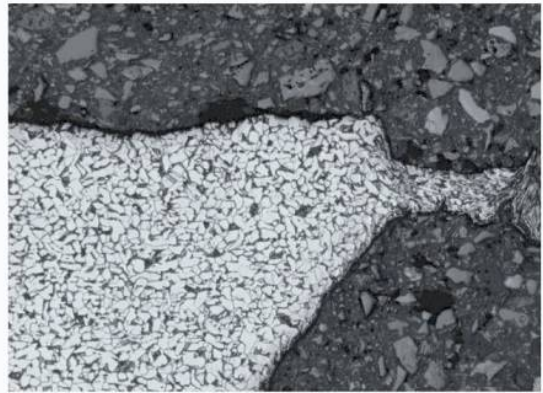
Fig. 2 — Metallographic cross section sample F1. 100X 2% Nital etch.
